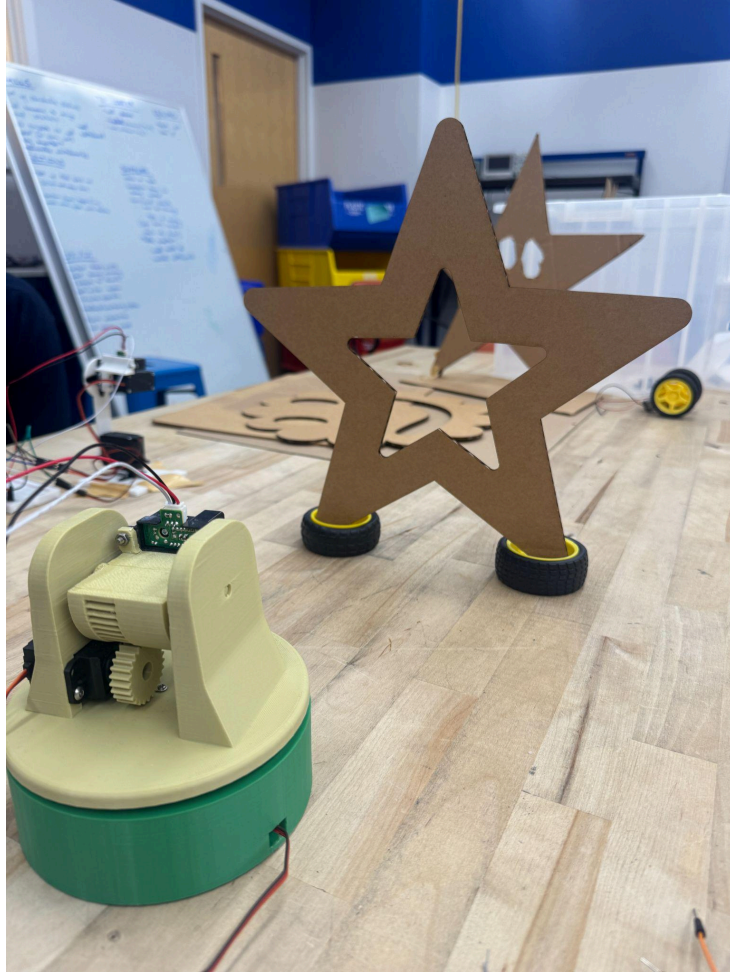
Fig 13: Image of the single servo scan setup.
